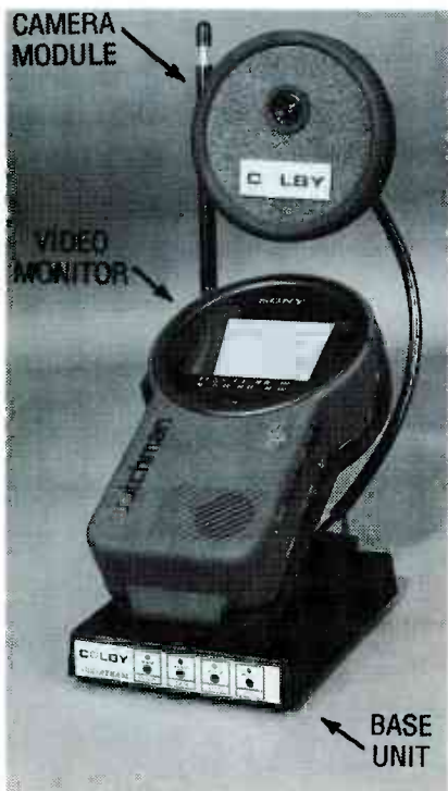
FIG. 1—THE VIDEOPHONE CONSISTS OF THREE SECTIONS: the CCD camera module at the top, the video monitor, and the base unit that contains the videophone circuitry.
