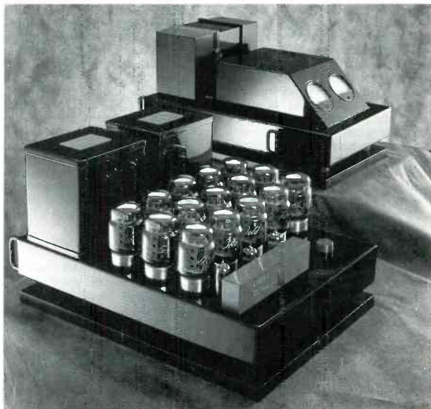
FIG. 1—THE CARVER SILVER SEVEN POWER AMPLIFIER can deliver 375 watts into an 8-ohm speaker load from 20 Hz to 20 kHz with less than 0.5% total harmonic distortion.
